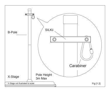
The SILKii should be installed at the top of the pole – over the X-Joint Hex Key hole - this could be done before the B-Pole is attached to the A-Pole, or a ladder will be needed. When installing on an X-STAGE, it is advisable to remove the B-Pole, then install the SILKii, before replacing the B-Pole. Additional weight is mandatory.
