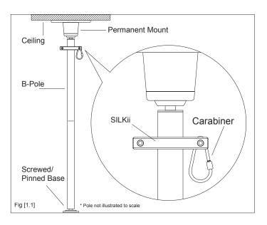
The SILKii can be installed at the top of an XPERT or SPORT pole that is mounted using a permanent fixing or on an X-Stage. SILKii MUST NOT be used on a stand-alone pole that is not secured using a permanent fixing/ceiling plate/mount or a secured base.
