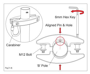
Attach the side with the pin to the pole. Once the pin has fully engaged with the hole. Line up the other half of the SILKii with the 2 x M12 bolts and fasten securely. Tighten screws progressively. If you tighten one screw too quickly, this will lock one side of the SILKii. Once correctly fastened, the SILKii is now in place and the Carabiner(s) can now be attached.
