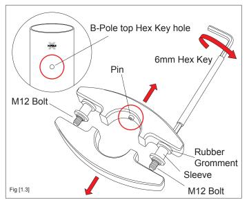
Remove the 2 x M12 bolts on either side of the SILKii – note the pin on one side of the SILKii. The pin locates into the Hex Key hole at the top of the B-POLE. Undo each side evenly otherwise the SILKii will lock. Whilst loosening the screws, please ensure that they are not completely removed from the SILKii unit.
